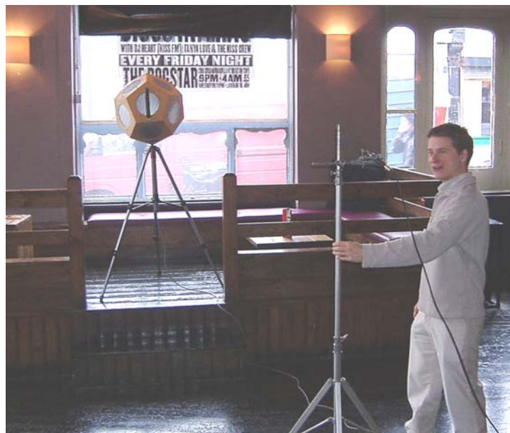
Figure 4.2 – Photo of the source and receiver placed in their first positions
