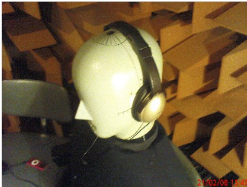
Figure 22 – Binaural head with Bose headphones in place
